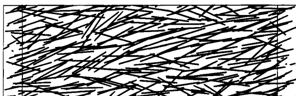
Figure 3. Configuration of LC monomer at T^* = 2 . The phase is nematic. The cell is viewed from a direction defined by the intersection of the XZ plane and the plane perpendicular to the director orientation.
