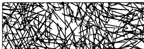
Figure 7. Configuration at T^* = 3 (projected on the XY plane) at a monomer conversion of 86%. Drawing conventions are as in Figure 2.
